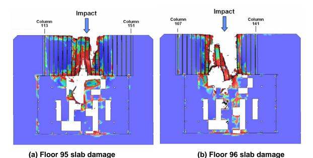
Figure E-41. More severe impact damage to the slabs on 1 floors 95 and 96 of WTC 1 (plan view).
