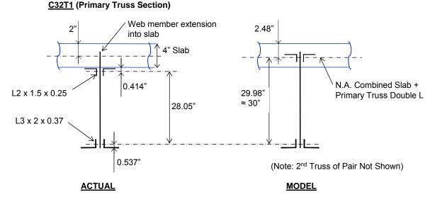
Figure 2–18. Typical primary truss cross-section, as-designed and as-modeled.
