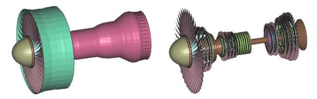
Figure E-17. Pratt & Whitney PW4000 turbofan engine model.
