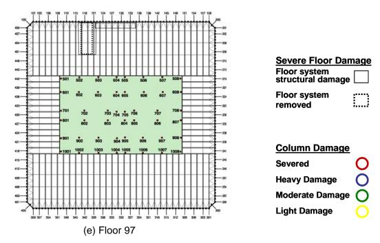
Figure 7–12. Summary of the floor-by-floor structural damage to the floors and columns of WTC 1 (base case) (continued).
