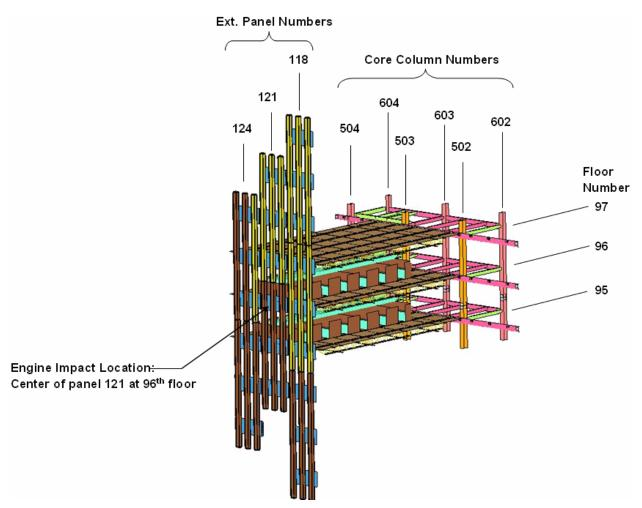
Figure 5-60. Tower subassembly model.
