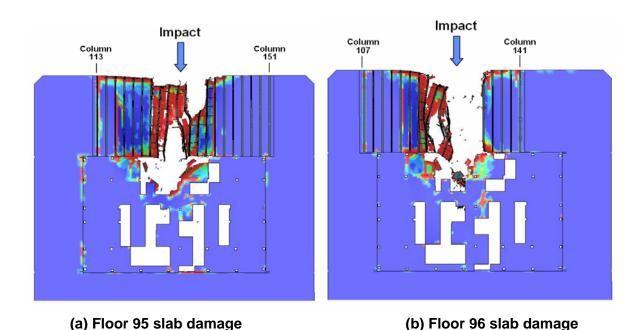
Figure 7–11. Base Case impact damage to the slabs on floors 95 and 96 of WTC 1 (plan view).
