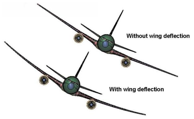
Figure 5-32. Boeing 767-200ER model wing deflections.
