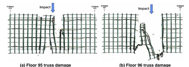
Figure E-40. More severe impact damage to the trusses on floors 95 and 96 of WTC 1 (plan view).
