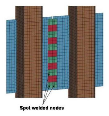
Figure 5–4. Model of the spandrel splice plate connection.
