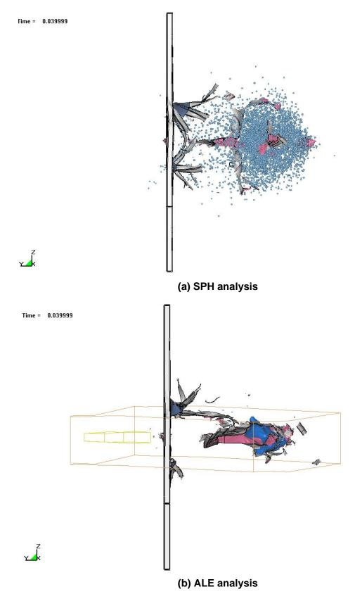
Figure 5–59. Side view of structural damage and fuel dispersion at 0.04 s.
