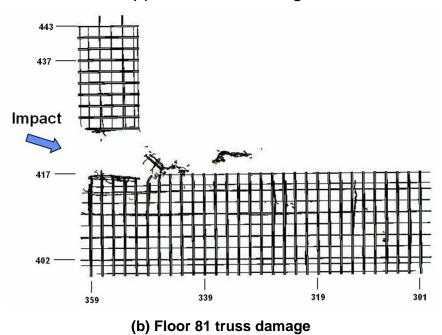
Figure 7–40. Base case impact damage to the trusses on floors 80 and 81 of WTC 2 (plan view).
