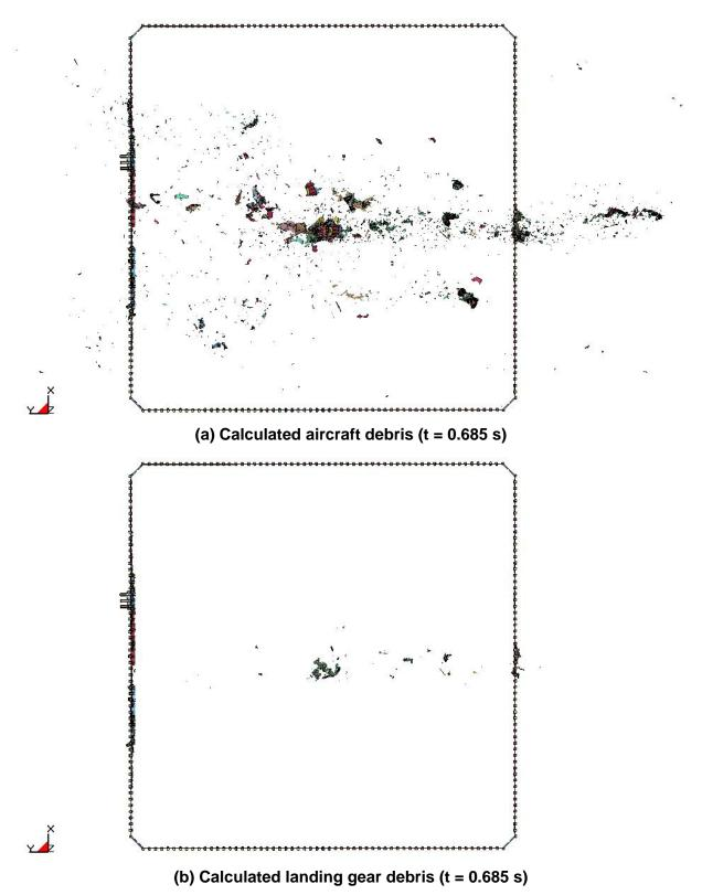
Figure 7–67. More severe damage aircraft debris distribution in WTC 1.
