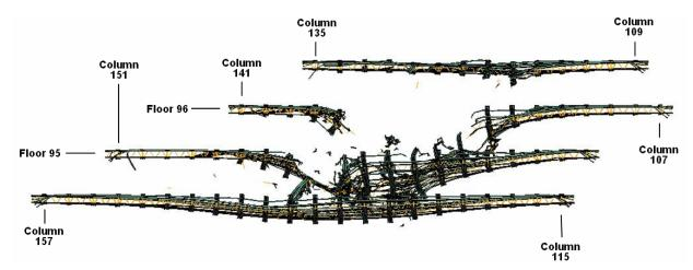
Figure E-39. Calculated more severe impact damage to the WTC 1 floor trusses (front view).
