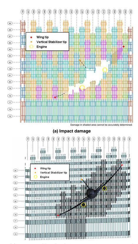
(b) Impact conditions (vertical angle =  $6^{\circ}$ , lateral angle =  $13^{\circ}$ ) Figure E–24. WTC 2 impact conditions and the impact pattern.
