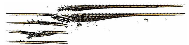
Figure E-57. Calculated more severe impact damage to the WTC 2 floor trusses (front view).
