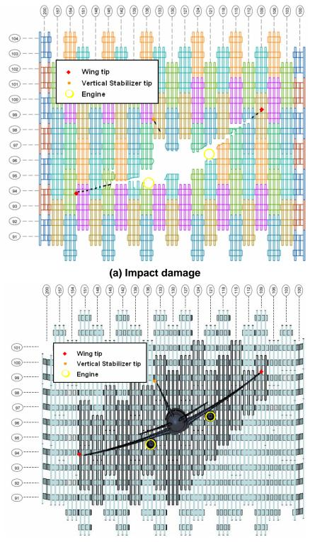
(b) Impact conditions (vertical angle =  $10.6^{\circ}$ , lateral angle =  $0^{\circ}$ ) Figure E-23. WTC1 impact conditions and the impact pattern.
