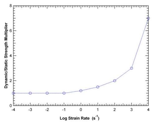
Figure 5-29. Tabular concrete strain rate effects curve.
