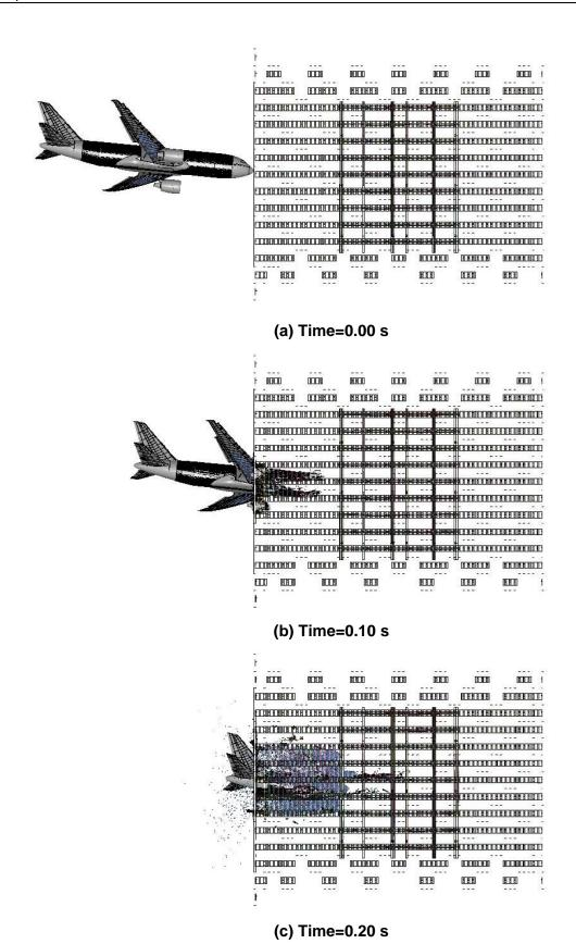
Figure 7-18. WTC 1 more severe global impact analysis (side view).
