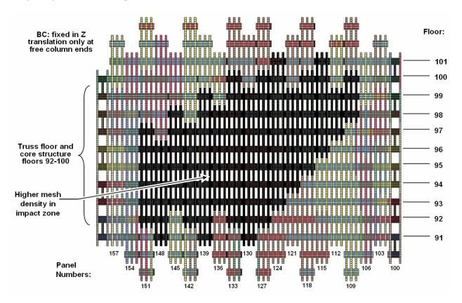
Figure 5–2. Impact face of the WTC 1 global model, floors 91–101.
