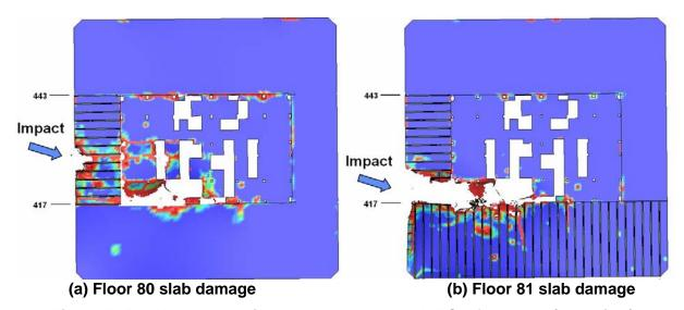
Figure E-59. More severe impact damage to the WTC 2 floor slab (plan view).
