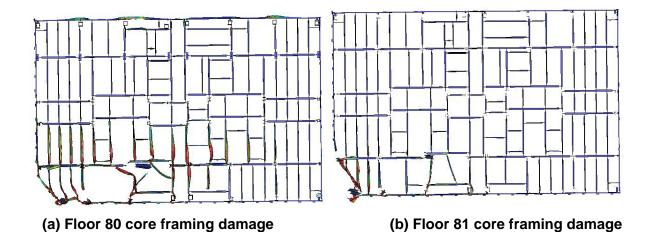
Figure 7–38. Base case impact damage to the core beams of floors 80 and 81 of WTC 2.
