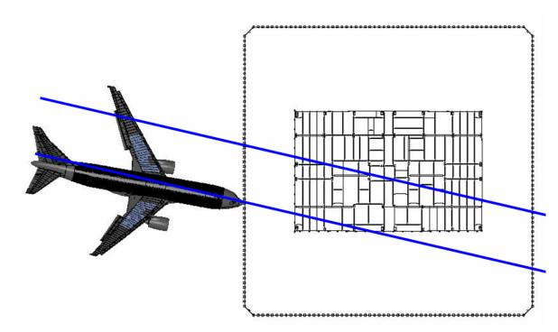
Figure 7–84. Projected debris path for the WTC 2 north face cold spot.
