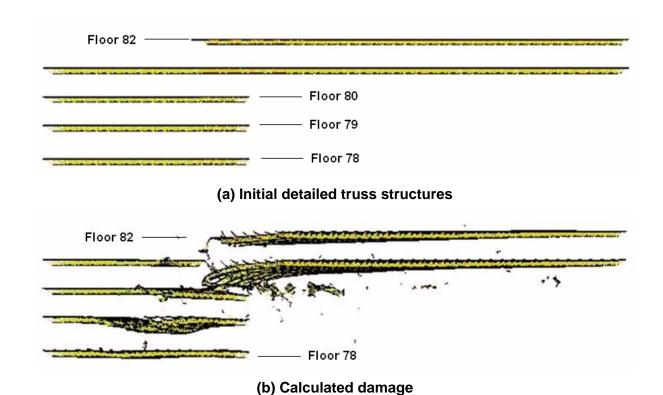
Figure E-49. Base case impact damage to the WTC 2 floor trusses (front view).
