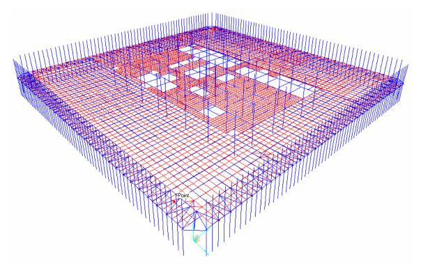
Figure E-4. Typical beam-framed floor model (floor 75 of WTC 2).
