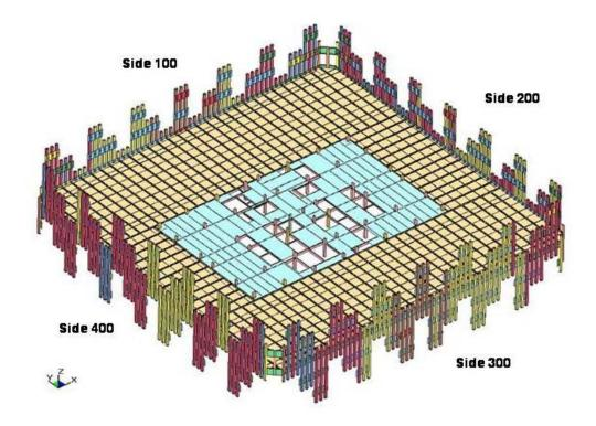
Figure 5-16. Detailed model of floor 96 of WTC 1.
