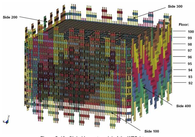
Figure 5–18. Global impact model of the WTC 1 tower.
