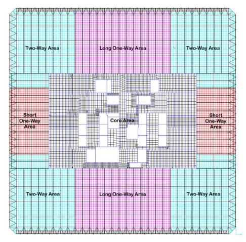
Figure 2–16. Typical floor truss framing zones.
