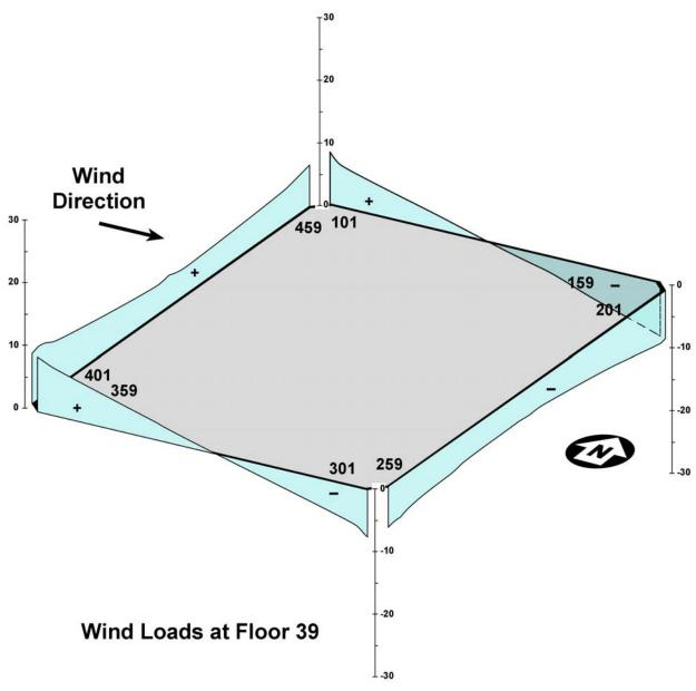
Figure 4–7. Three-dimensional distribution of normal stresses in the exterior walls of WTC 1 due to original WTC wind loads only at floors B6 and 39 (continued).
