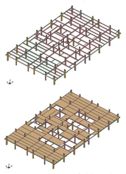
Figure 5–9. Model of the core of floor 96 of WTC 1 (with and without floor slab).
