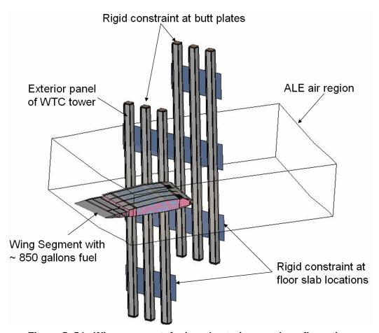
Figure 5-54. Wing segment, fuel, and exterior panel configuration.
