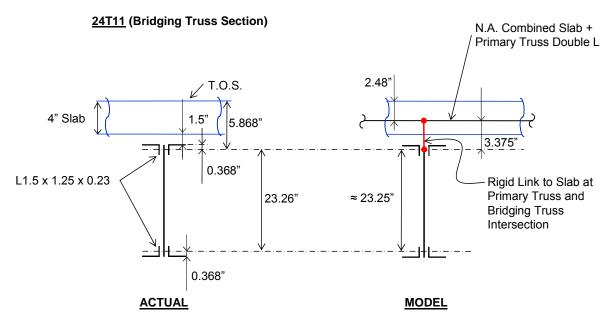
Figure 2–19. Typical bridging truss cross–section, as-designed and as-modeled.
