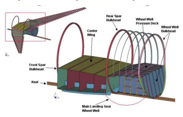
Figure 5–38. Integration of the fuselage and wing structures.
