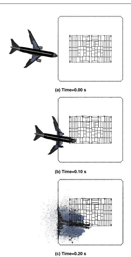
Figure 7–34. WTC 2 base case global impact analysis (plan view).
