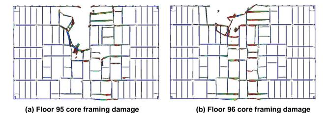
Figure E–38. More severe impact damage to the core beams of floors 95 and 96 of WTC 1.
