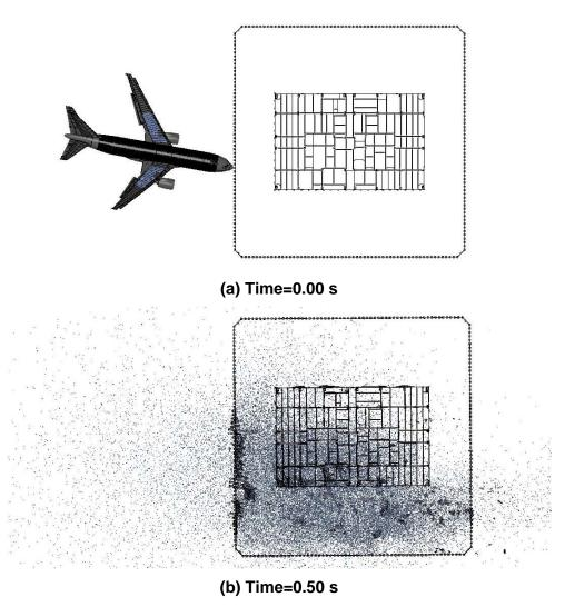
Figure E-45. WTC 2 base case global impact analysis – plan view.
