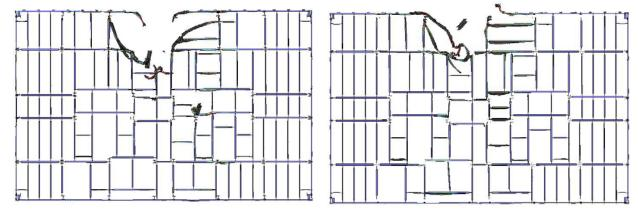
(a) Floor 95 core framing damage
