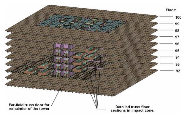
Figure 5–19. Interior structures and contents of the WTC 1 global impact model.
