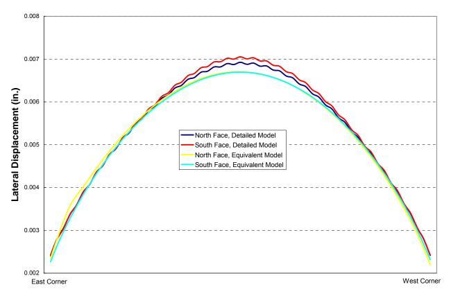
Figure 2–14. Deflections of the north and south faces of the floor for the detailed and equivalent floor models.
