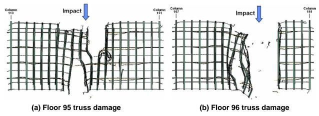
Figure E-32. Base case impact damage to the trusses on floors 95 and 96 of WTC 1 (plan view).
