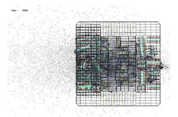
Figure E-43. Calculated fuel distribution and debris damage in the more severe WTC 1 analysis.
