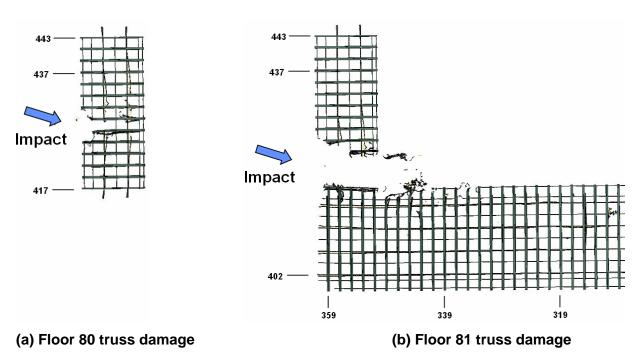
Figure E-58. More severe impact damage to the trusses on floors 80 and 81 of WTC 2 (plan view).
