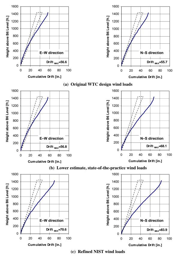
Figure 4–1. Cumulative drift diagrams for WTC 1 under the three wind loading cases.
