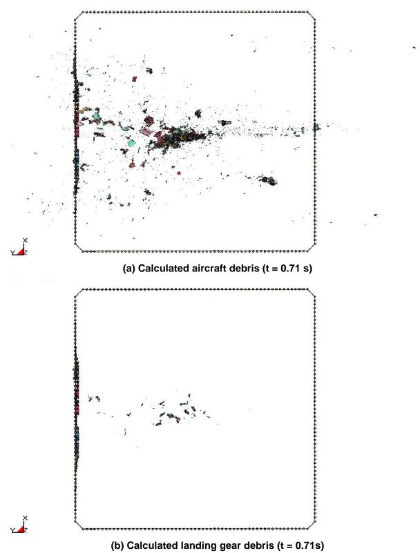
Figure 7–66. Base case aircraft debris distribution in WTC 1.
