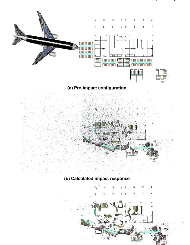
(c) Calculated impact response (fuel removed)
