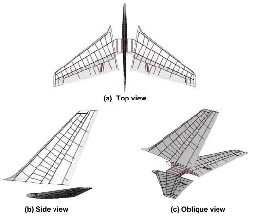
Figure 5-33. Empennage model of the 767-200ER aircraft.
