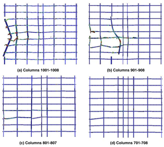
Figure E-47. Base case impact damage to the WTC 2 core columns.
