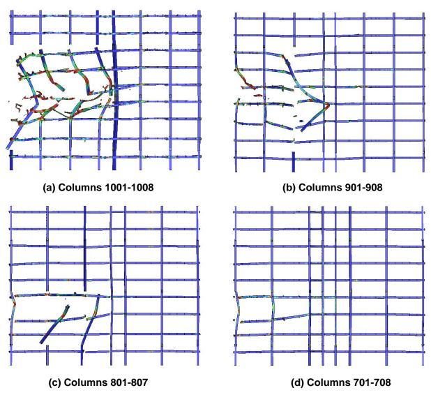
Figure E-55. More severe impact damage to the WTC 2 core columns.
