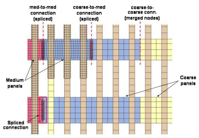
Figure 5–5. Placement of spandrel splice plates in the exterior wall model.
