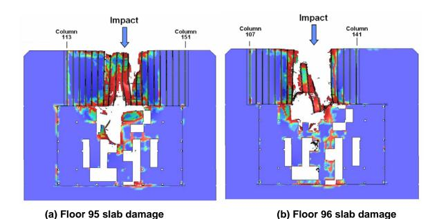
Figure 7–25. More severe impact damage to the slabs on floors 95 and 96 of WTC 1 (plan view).
