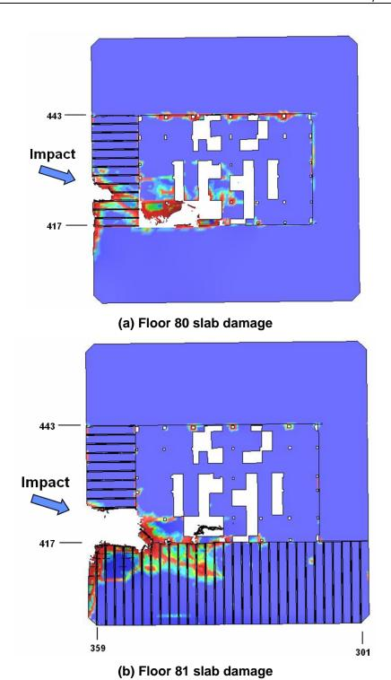
Figure 7–41. Base case impact damage to the slabs on floors 80 and 81 of WTC 2 (plan view).
