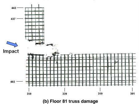
Figure 7–54. More severe impact damage to the trusses on floors 80 and 81 of WTC 2 (plan view).
