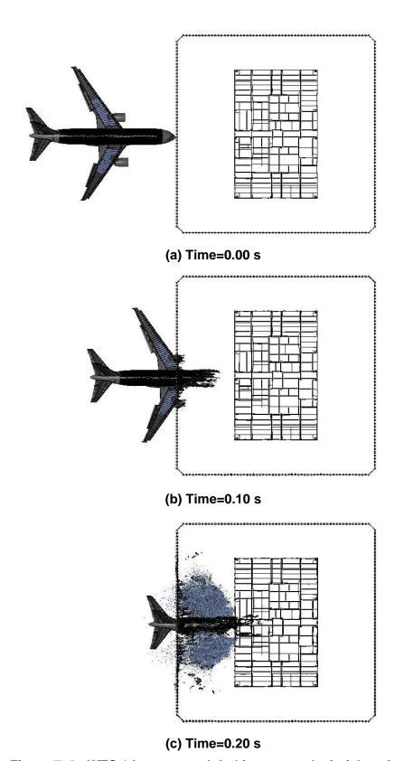
Figure 7–3. WTC 1 base case global impact analysis (plan view).
