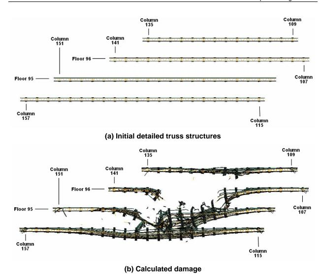
Figure 7–23. More severe impact damage to the WTC 1 floor trusses (front view).
