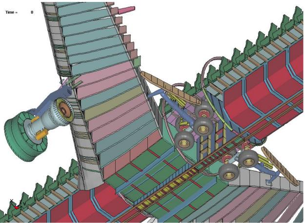
Figure 5–35. Underside of the 767 airframe model (skin removed) showing retracted landing gear, engine, and ULDs.
