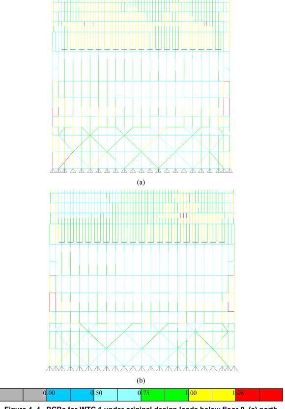
Figure 4–4. RCRs for WTC 1 under original design loads below floor 9, (a) north elevation, and (b) east elevation.
