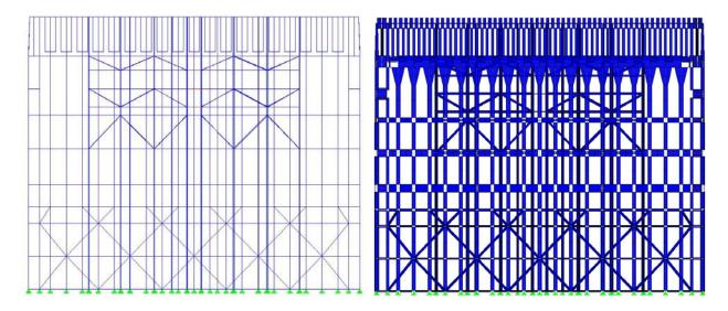
Figure 2-3. Frame view and rendered view of the WTC 1 model (foundation to floor 9).
