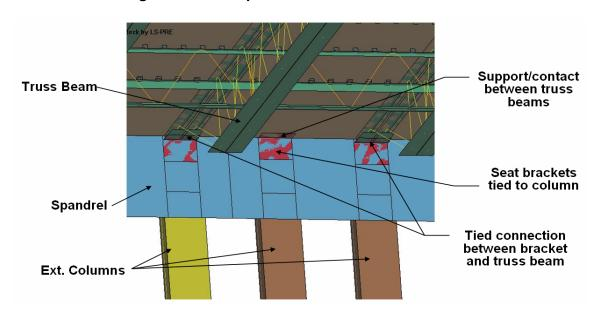
Figure 5–14. Truss floor connection detail at exterior wall.
