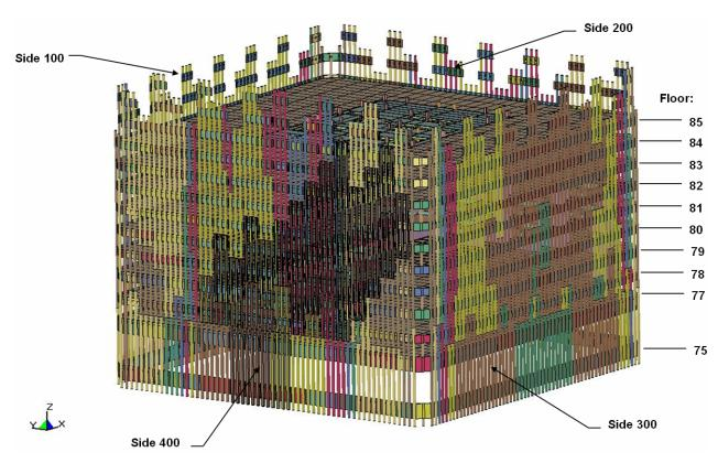
Figure 5-21. Global impact model of the WTC 2 tower.
