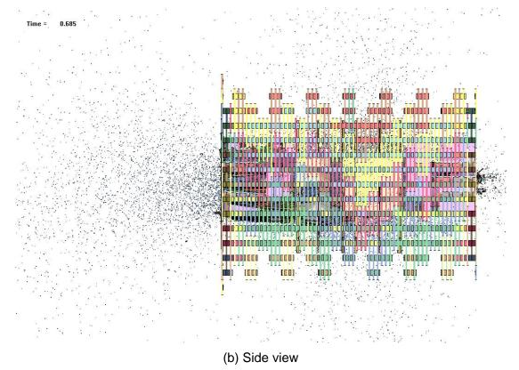
Figure 7–28. Calculated fuel distribution in the more severe WTC 1 analysis.
