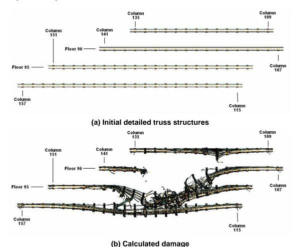
Figure E–31. Base case impact damage to the WTC 1 floor trusses (front view).
