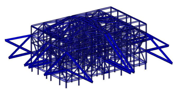
Figure 2–11. Rendered 3–D model of the WTC 1 hat truss.
