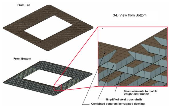
Figure 5-13. Simplified far field truss floor model.
