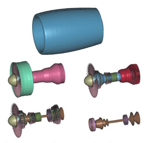
Figure 5-42. Pratt & Whitney PW4000 turbofan engine model.
