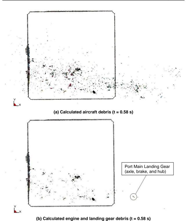
Figure 7–79. Aircraft debris distribution in the more severe WTC 2 impact.
