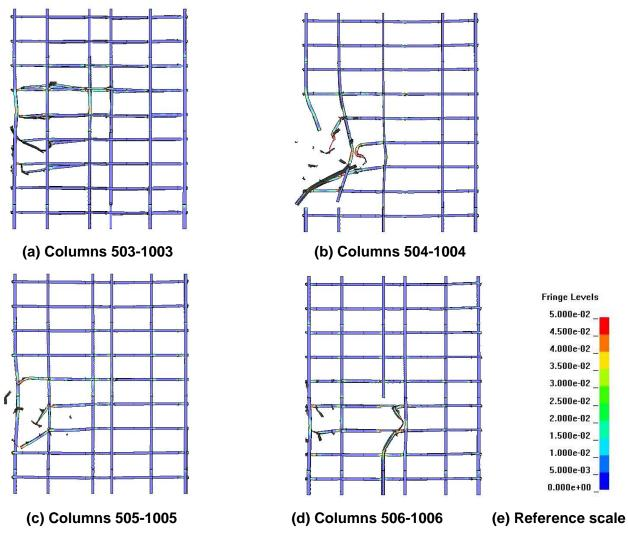
Figure 7–6. Base case impact damage to the WTC 1 core columns.
