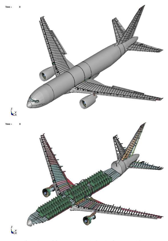
Figure 5–30. Finite element model of the Boeing 767-200ER.
