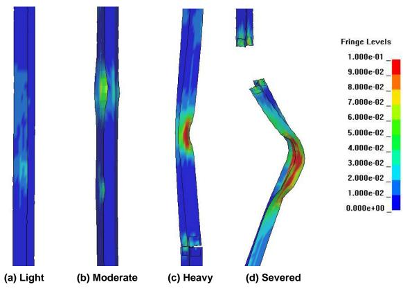
Figure 7–7. Classification of damage levels in core columns.
