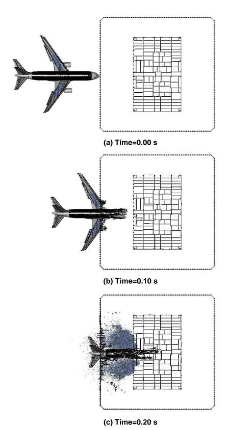
Figure 7–19. WTC 1 more severe global impact analysis (plan view).
