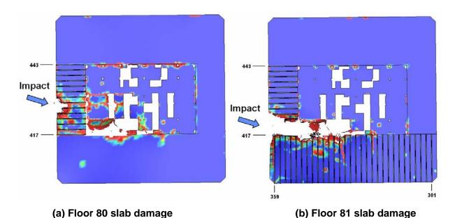
Figure 7-55. More severe impact damage to the WTC 2 floor slab (plan view).
