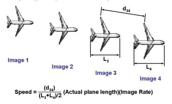
Figure 6–3. Simplified motion analysis procedure to determine aircraft speed.
