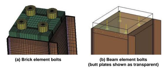
Figure 5-46. Modeling of exterior column bolted connection.
