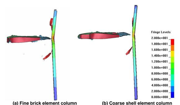
Figure 5–45. Exterior column response comparison, showing contours of the displacement magnitude (in.).
