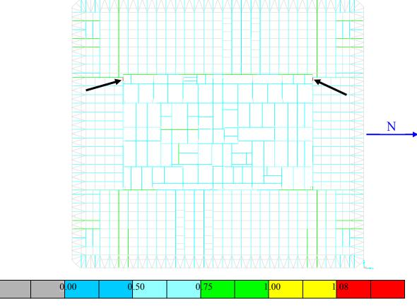
Figure 4–9. DCRs for the typical beam-framed floor under original WTC design criteria loading.
