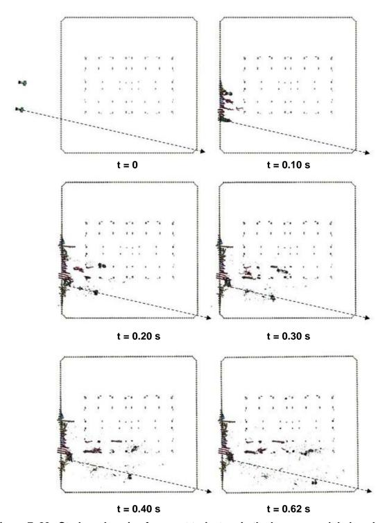
Figure 7–80. Starboard engine fragment trajectory in the base case global analysis of WTC 2.
