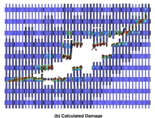
Figure 7–20. More severe impact damage to the WTC 1 exterior wall.
