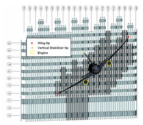
Figure 6–9. Orientation and trajectory of UAL 175 that matches the impact pattern (vertical approach angle = 6°, lateral approach angle = 17°).
