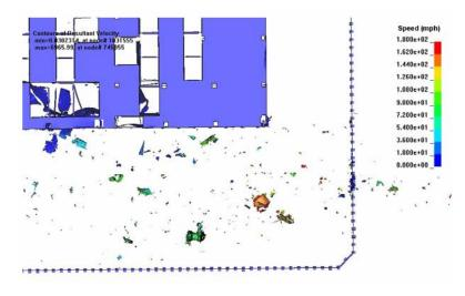
(c) Residual speed of aircraft debris (contours in mph)
