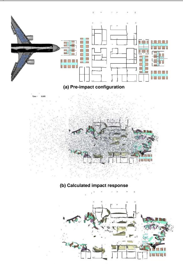
(c) Calculated impact response (fuel removed)
