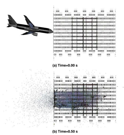
Figure E-26. WTC 1 base case global impact analysis - side view.
