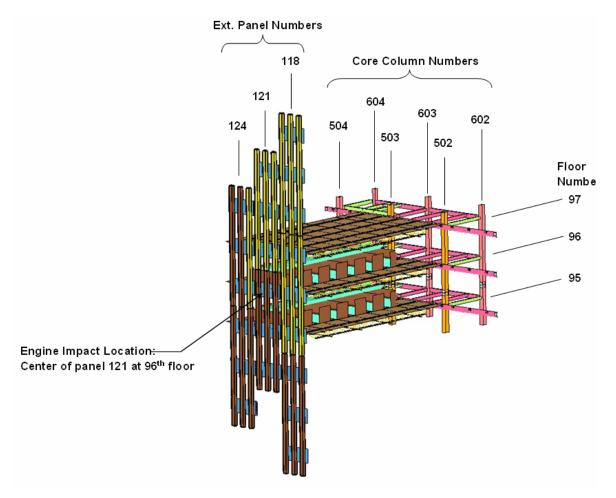
Figure E-21. Final WTC tower subassembly model.
