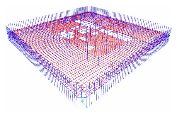
Figure 2–21. Typical beam-framed floor model (floor 75 of WTC 2).
