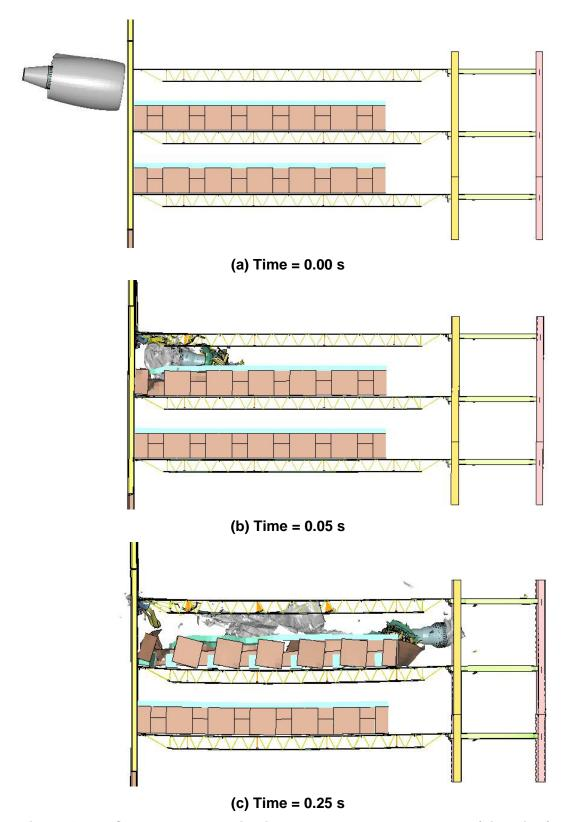
Figure 5–62. Subassembly-engine impact and breakup response (side view).
