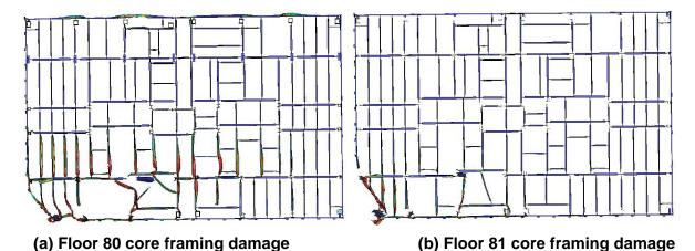
Figure E-48. Base case impact damage to the core beams of floors 80 and 81 of WTC 2.
