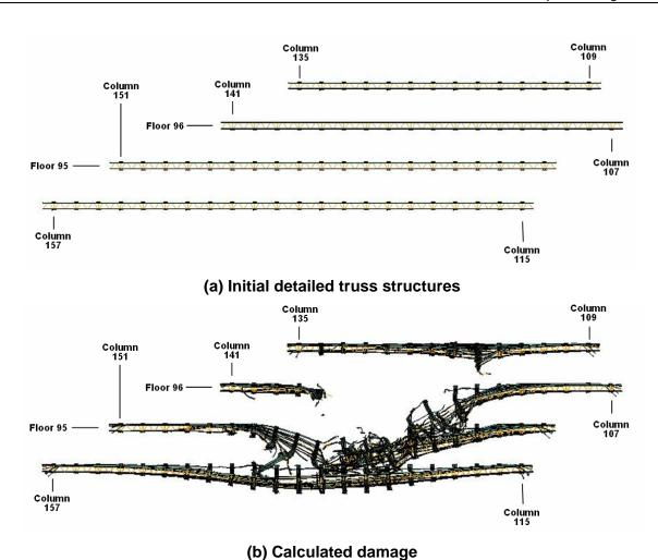
Figure 7–9. Base case impact damage to the WTC 1 floor trusses (front view).
