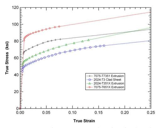
Figure 5–43. True stress-strain curves developed for various aircraft aluminum alloys.
