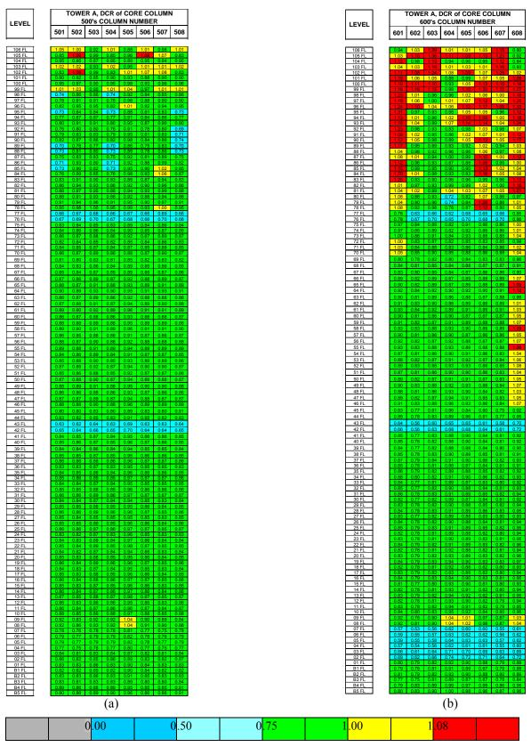
Figure 4–5. DCRs for WTC 1 core columns under original design loads, (a) 500 line, and (b) 600 line.
