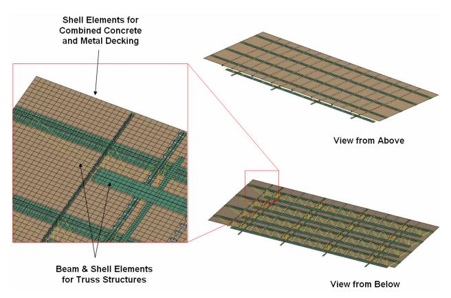
Figure 5-49. Simplified model of the truss floor system.
