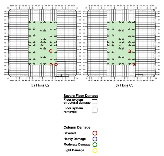
Figure 7–42. Summary of the floor-by-floor structural damage to the floors and columns of WTC 2 (base case) (continued).
