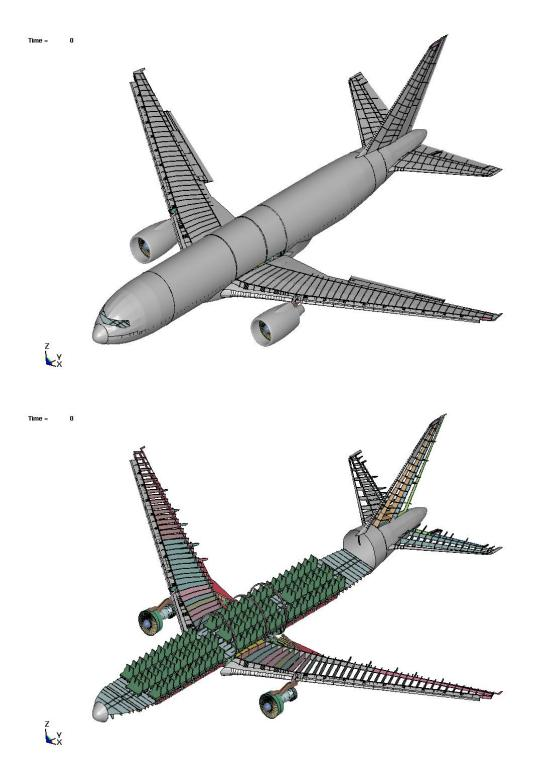
Figure E–16. Finite element model of the Boeing 767-200ER.
