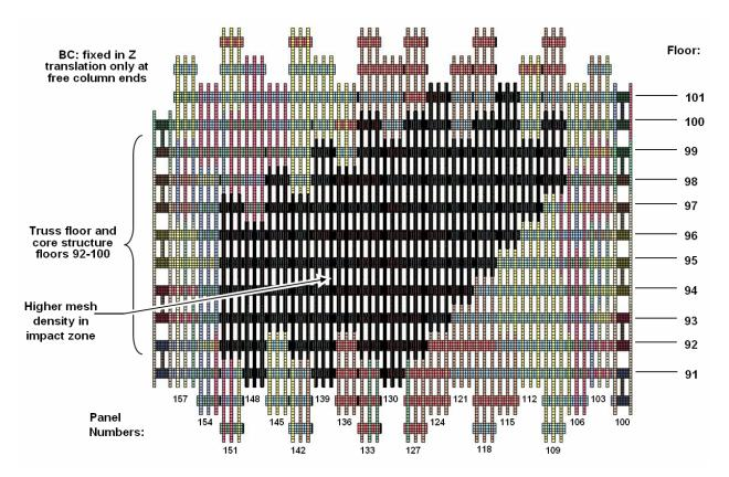
Figure E-7. Impact face of the WTC 1 model, floors 91-101.
