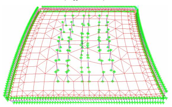
Figure 2–13. Deflection of equivalent floor model due to lateral loading (exaggerated scale).
