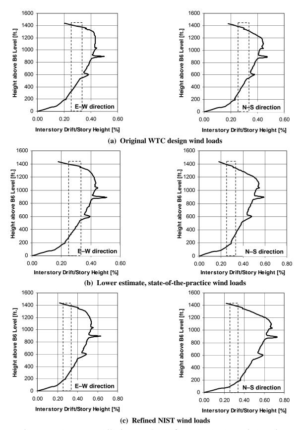
Figure 4–2. Inter-story drift diagrams for WTC 1 under the three wind loading cases.
