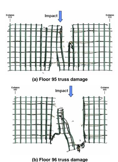
Figure 7–24. More severe impact damage to the trusses on floors 95 and 96 of WTC 1 (plan view).
