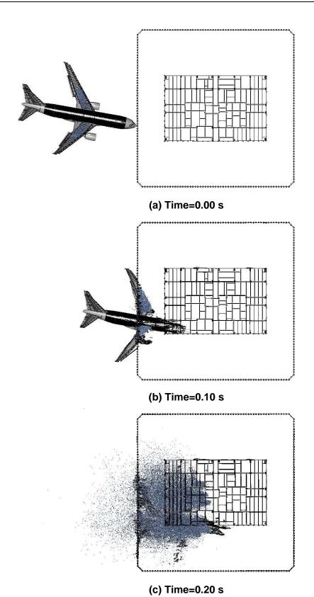
Figure 7–49. WTC 2 more severe global impact analysis (plan view).
