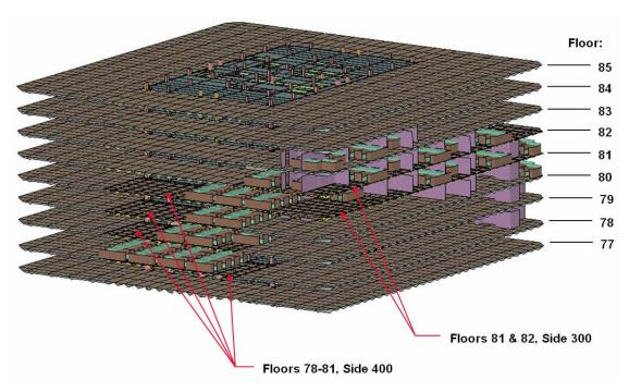
Figure 5–22. Interior structures and contents of the WTC 2 global impact model.
