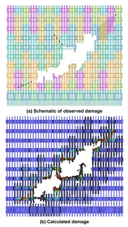
Figure 7-50. More severe impact damage to the WTC 2 exterior wall.
