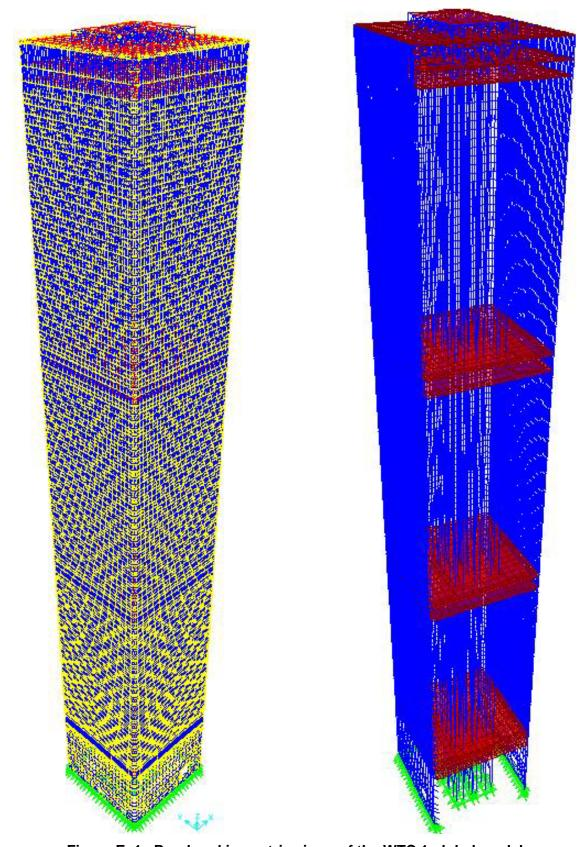
Figure E–1. Rendered isometric views of the WTC 1 global model.
