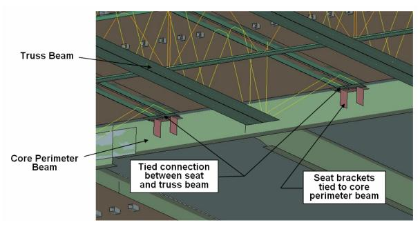
Figure 5-15. Truss floor connection detail at core perimeter.
