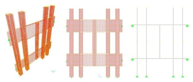
Figure 2-9. Shell element and frame models of typical exterior wall corner panel.
