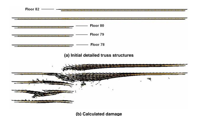
Figure 7–53. More severe impact damage to the WTC 2 floor trusses (front view).
