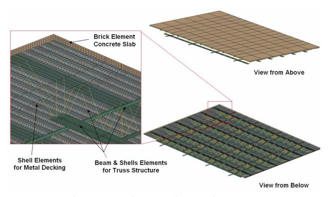
Figure 5–48. Detailed model of the truss floor system.
