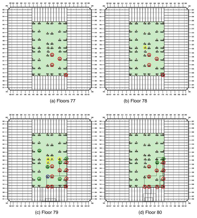
Figure 7–56. Summary of the floor-by-floor structural damage to the floors and columns of WTC 2 (more severe case).
