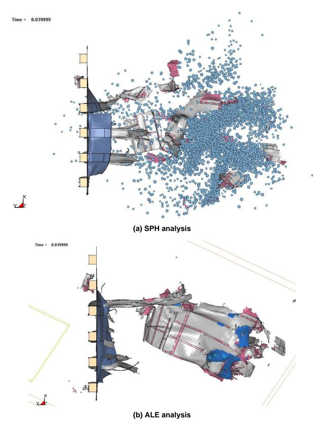
Figure 5-58. Top view of structural damage and fuel dispersion at 0.04 s.
