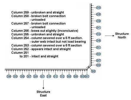
Figure 7–75. Documented damage to the northeast corner of floor 81 of WTC 2.
