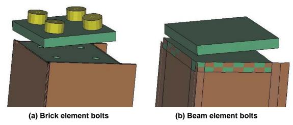
Figure 5–47. Failure comparison of exterior column bolted connection treatments.
