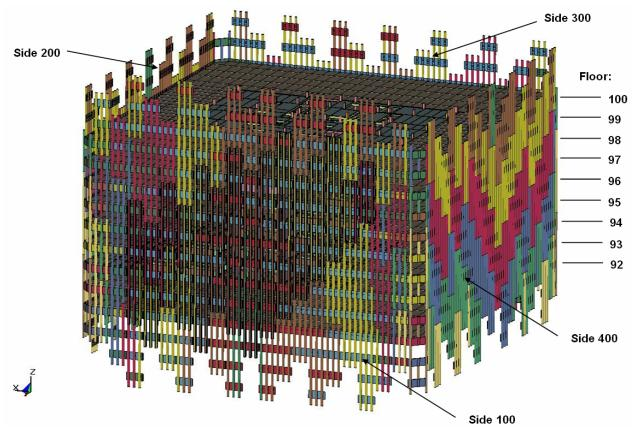
Figure E-11. Multi-floor global impact model of the WTC 1 tower.
