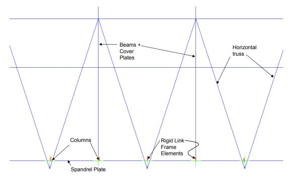
Figure 2–22. Horizontal truss modeling, slab not shown.
