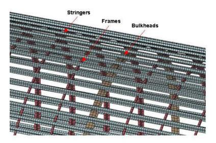
Figure 5–37. Model of fuselage interior frame and stringer construction.
