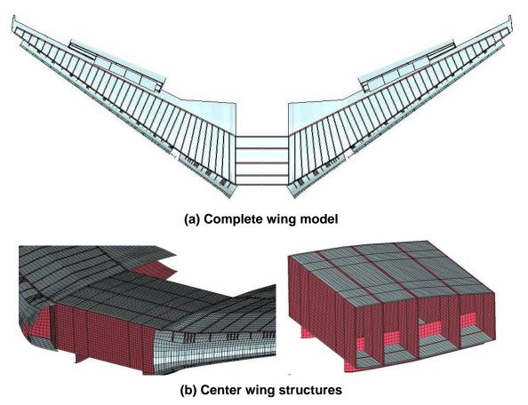
Figure 5–36. Complete wing structures for the 767 aircraft model.
