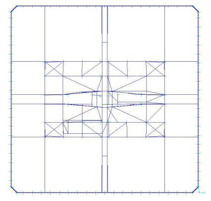
Figure 2–10. As-modeled plan of the WTC 1 hat truss.
