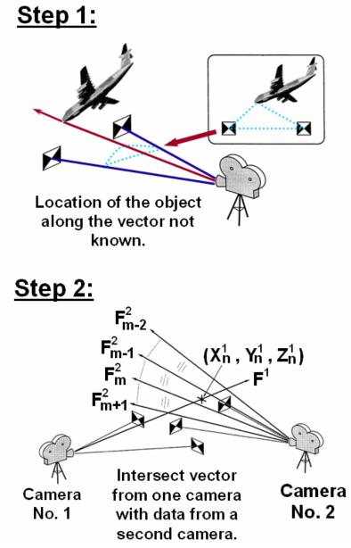
Figure 6–2. Complex motion analysis to measure object motions using multiple cameras.
