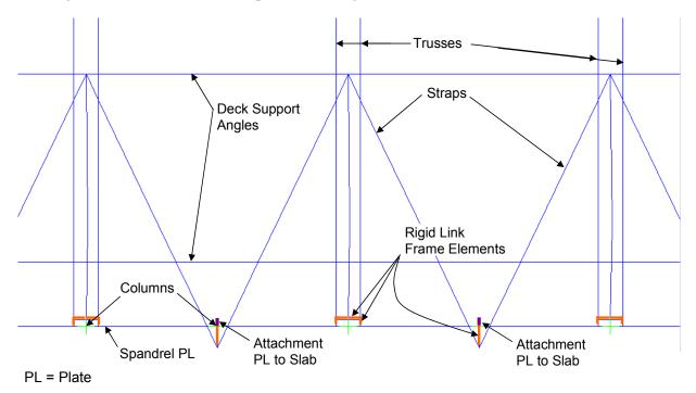
Figure 2–20. Strap anchors modeling, slab not shown.
