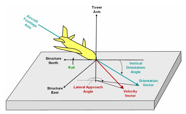
Figure 6–1. Definition of the aircraft impact parameters.
