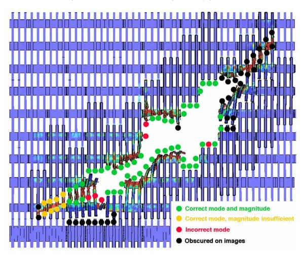
Figure 7–73. Comparison of observable and calculated base case impact damage to the south wall of WTC 2.
