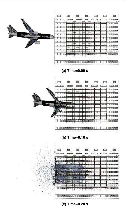
Figure 7-48. WTC 2 more severe global impact analysis (side view).
