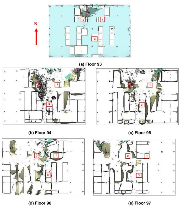
Figure 7-71. Base case stairwell disruption in WTC 1.
