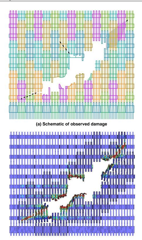
(b) Calculated damage Figure E-46. Base case impact damage to the WTC 2 exterior wall.
