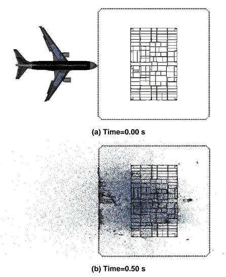
Figure E-27. WTC 1 base case global impact analysis – top view.
