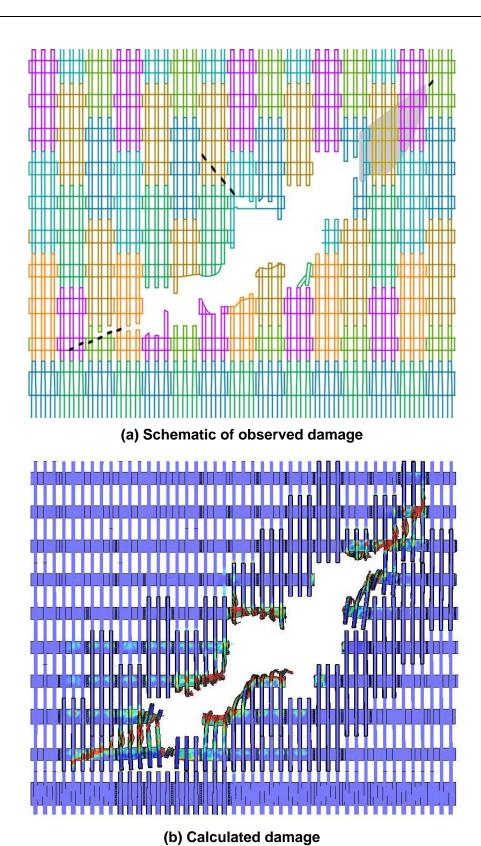
Figure 7–36. Base case impact damage to the WTC 2 exterior wall.
