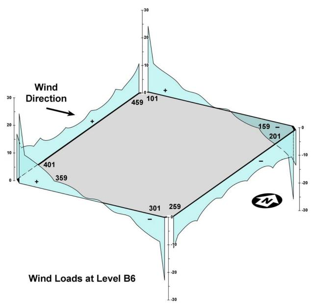
Figure 4–7. Three-dimensional distribution of normal stresses in the exterior walls of WTC 1 due to original WTC wind loads only at floors B6 and 39.
