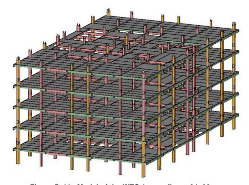
Figure 5-11. Model of the WTC 1 core, floors 94-98.
