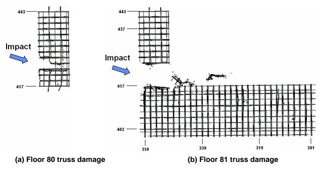
Figure E-50. Base case impact damage to the trusses on floors 80 and 81 of WTC 2 (plan view).
