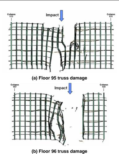
Figure 7–10. Base case impact damage to the trusses on floors 95 and 96 of WTC 1 (plan view).
