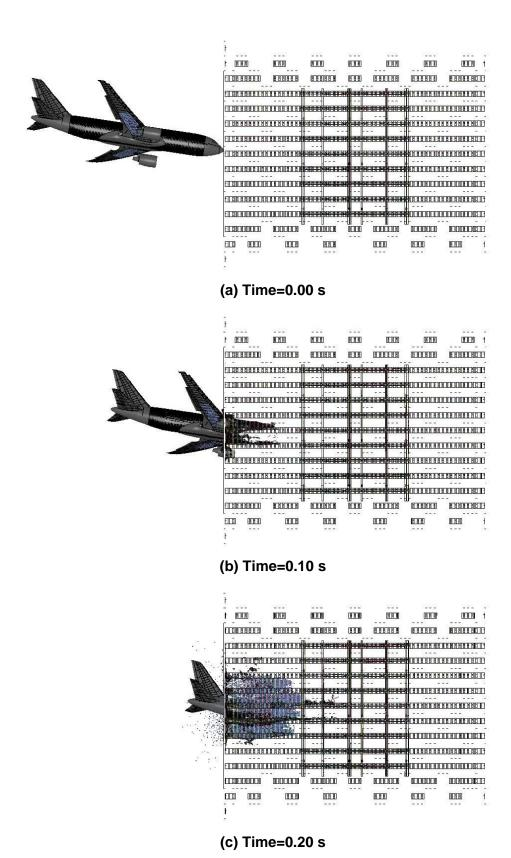
Figure 7–2. WTC 1 base case global impact analysis (side view).
