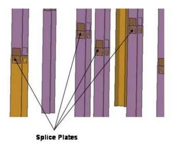
Figure 5-7. Detail of wide flange core columns splices
