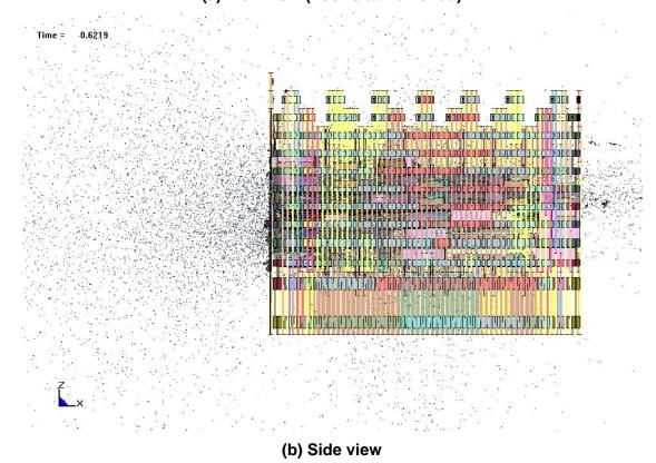
Figure 7–44. Calculated fuel distribution in the base case WTC 2 analysis.
