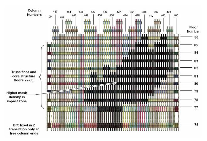
Figure 5–3. Impact face of the WTC 2 global model, floors 75–86.
