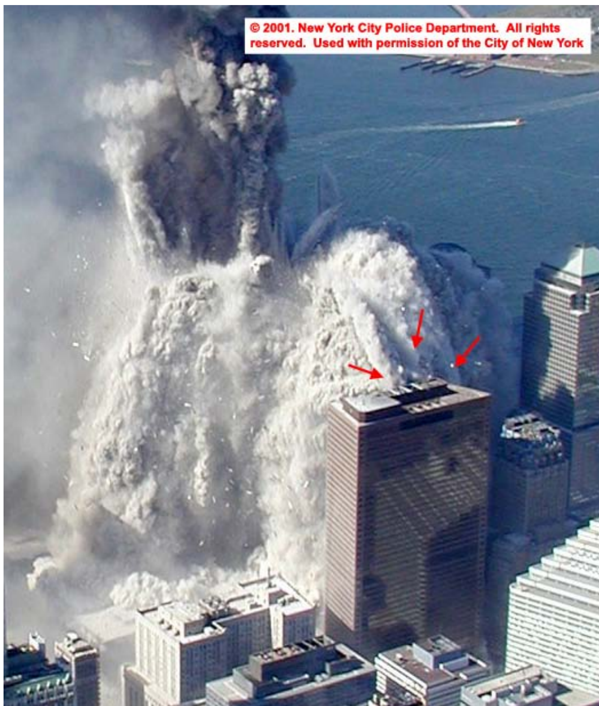
Figure 5–42. Aerial photograph shot 14\text{ s} \pm 0.5\text{ s} after WTC 1 began to collapse. Arrows mark arcs formed by debris that seemed to be ejected outwards from the debris cloud.
