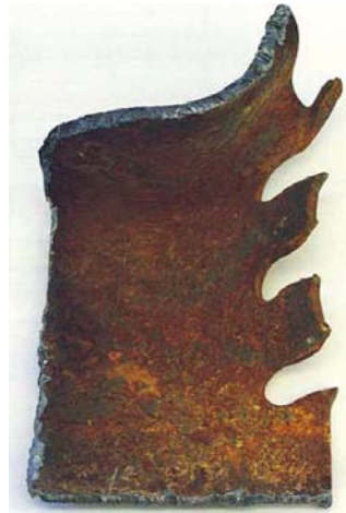
Figure 8–15. Steel samples recovered from WTC 5, showing tear-out of beam web.
