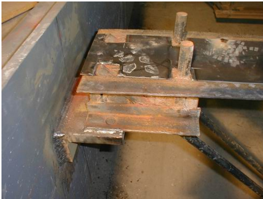
Figure 4–8. Restrained end condition of Assembly No. 1 prior to shimming.
