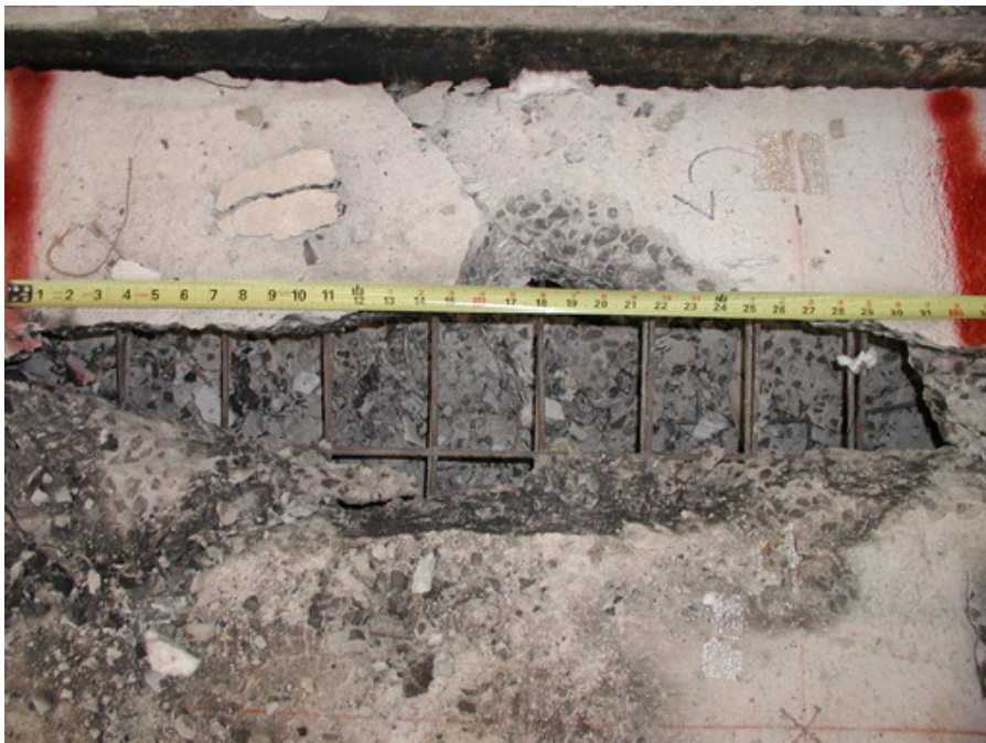
Figure 5–68. Unexposed surface of Assembly No. 4, close-up of concrete spalling on west side of assembly.
