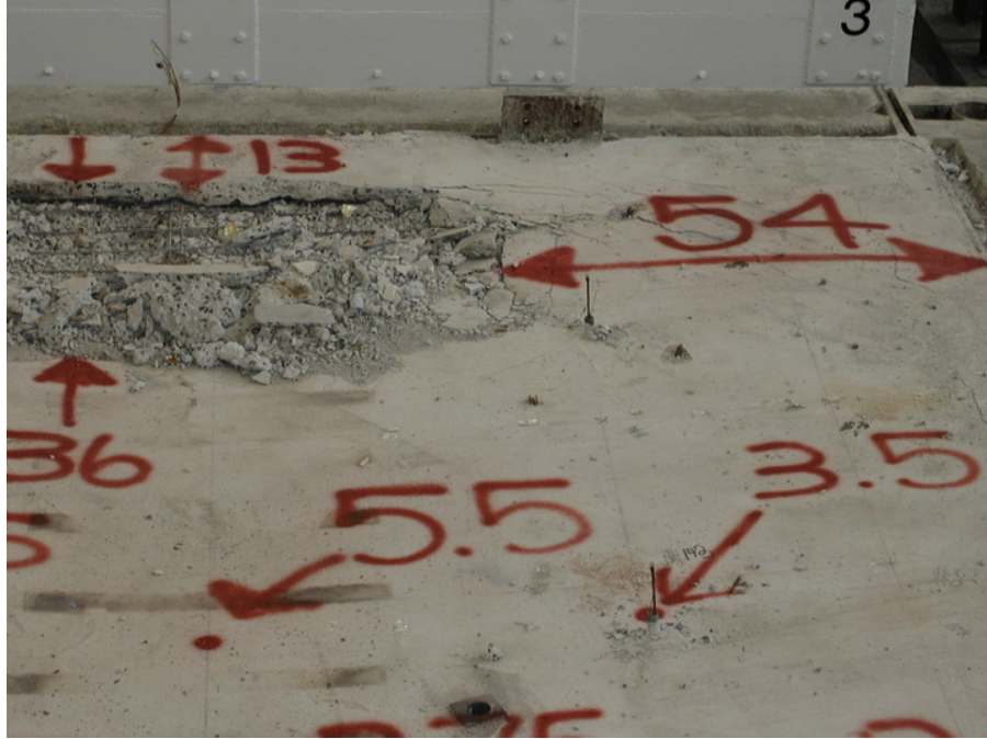
Figure 5–51. Detail of spalling concrete at north end of Assembly No. 3.
