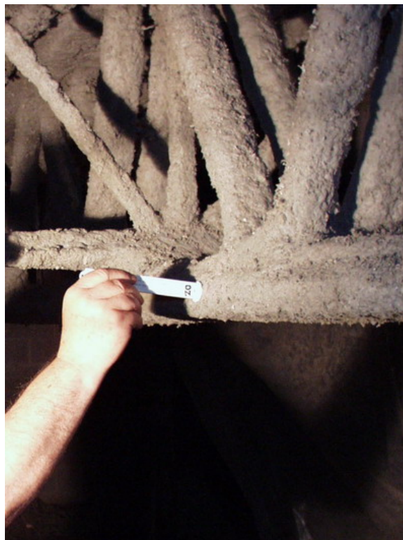
Figure 4-22. Measurement of SFRM thickness on truss chord.
