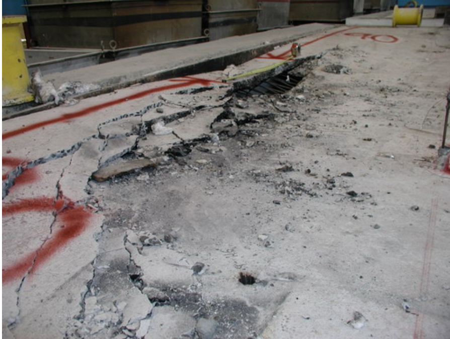
Figure 5–67. Unexposed surface of Assembly No. 4, view of concrete spalling on west side of assembly.
