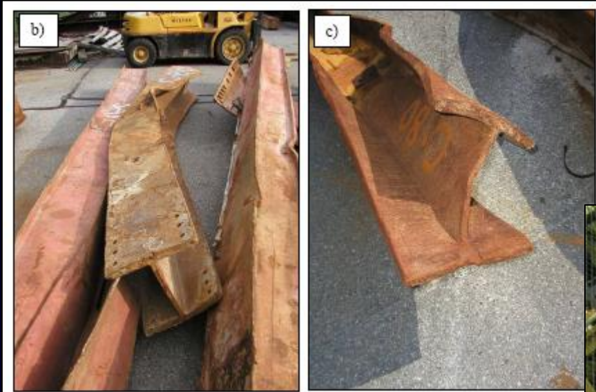
Figure 4-1, NCSTAR1-3C Core column from WTC 1 Floors 92-94
