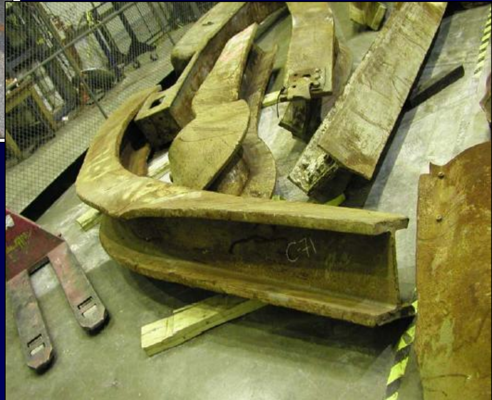
Figure 3-12e, NCSTAR1-3B Recovered core columns from WTC 1
