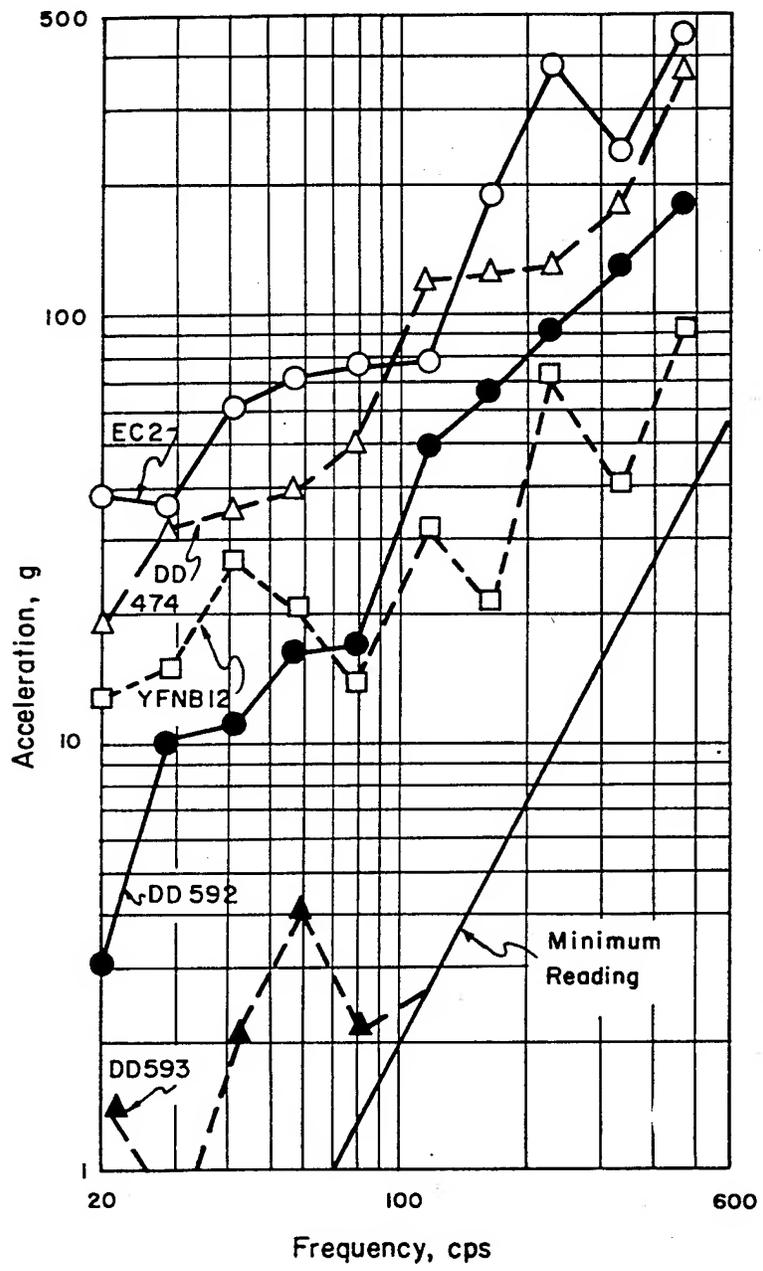
Figure 3.50 Shock spectra obtained near the bottom of a bulkhead on each of the surface targets, Shot Umbrella. Shock spectra are shown for Position 1 on EC-2, Position 17 on each of the three destroyers, and Position 2 on YFNB-12. On DD-593, deflections of the five highest-frequency reeds in the shock-spectrum recorder were all less than the minimum readable value.
