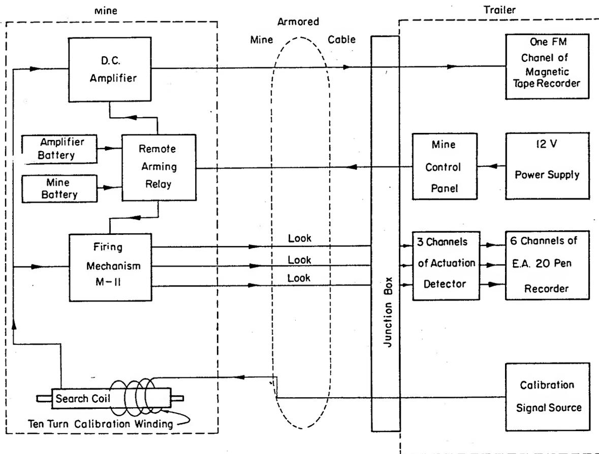
Figure 3.59 Block diagram of monitor system for mine Mark 25 Mod 0.
