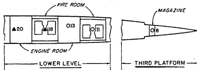
Figure 3.25 Location and designation of GTR stations on target destroyers.
