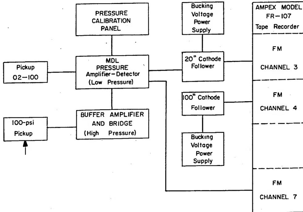
Figure 3.58 Block diagram of pressure measuring system.
