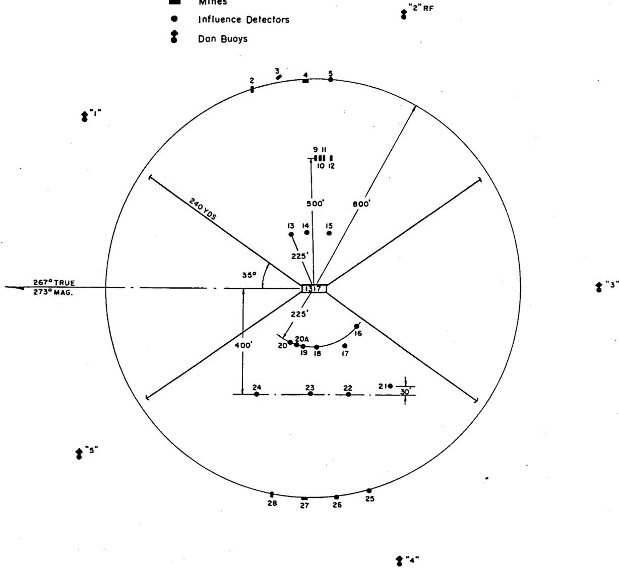
Figure 3.57 Schematic of underwater instrumentation and mines relative to Platform 1 (Station 681.01). For identification of code numbers of underwater units, see Table 3.12.
