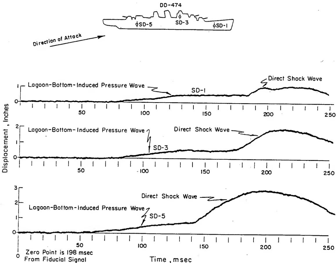
Figure 3.42 Vertical displacements on DD-474, Shot Umbrella.
