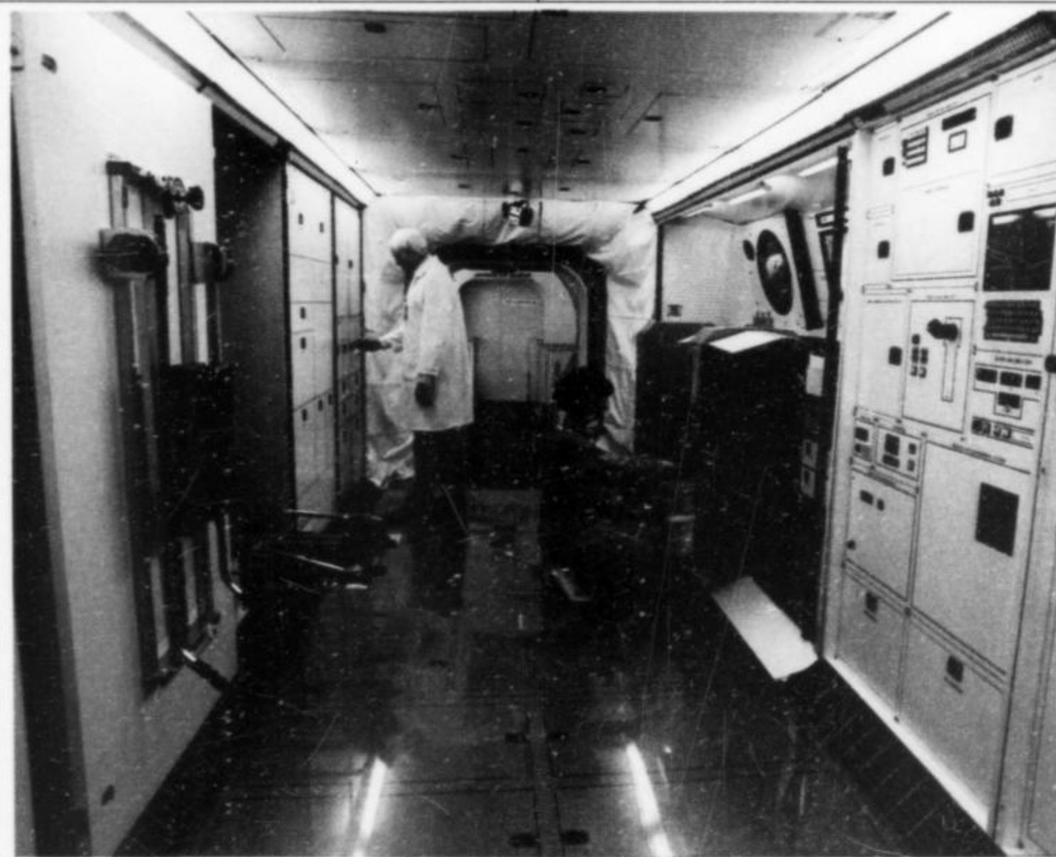
Interior of the U.S. habitat module has separate areas for sleeping and other activities. Astronauts would cook, exercise and perform other duties in the active zone, shown as arranged in the full-scale mockup at Marshall. Cross country skiing and rowing machines are visible.
