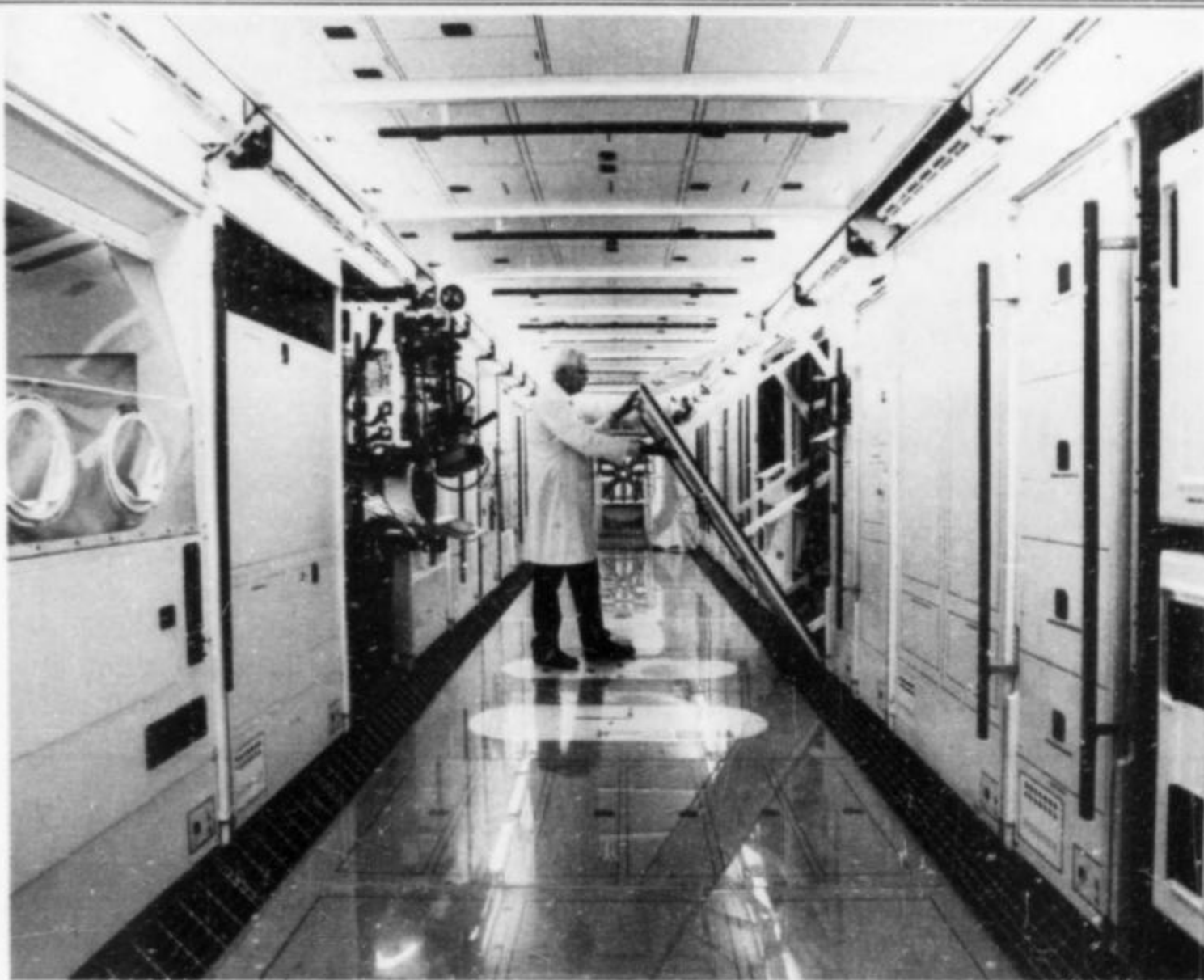
Interior of the station laboratory mockup includes experiment racks that can be pulled out for servicing, as the technician here is doing. Behind him is a small maintenance and repair shop. The laboratory would have stowage lockers above and below the rack areas on the walls.
