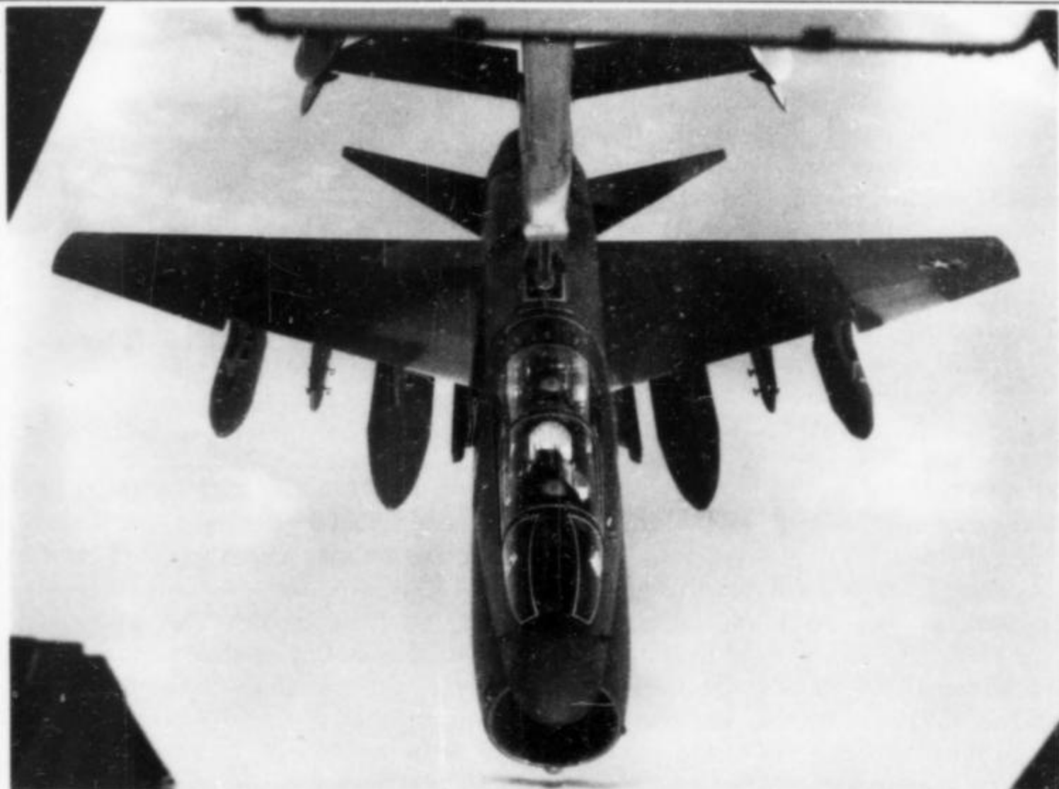
All USAF A-7 aircraft are limited to +5g with symmetrical wing stores like those shown on this two-seat A-7K undergoing aerial refueling. With asymmetrical stores, aircraft are limited to +4g.
