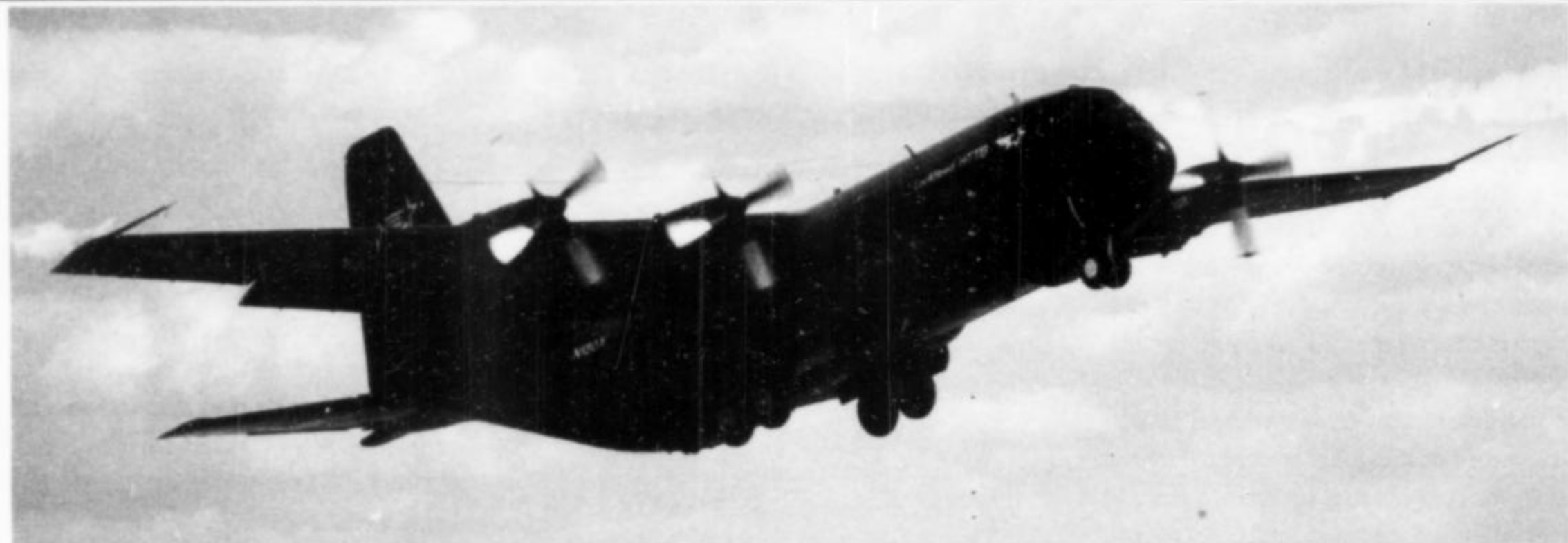
Lockheed C-130 HTTB demonstrator, equipped with Allison T56 Series 4 engines, is shown performing a STOL takeoff during a time-to-climb record attempt. The aircraft unofficially broke three STOL aircraft climb records and one weight-to-altitude mark on May 18 and 19.
