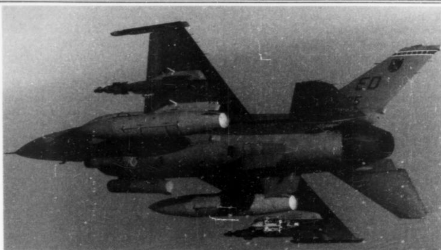
Full production of Martin Marietta Lantirn targeting pods, shown on board this F-16C, has been approved. Navigation pod production should reach 10 per month in 1989.
