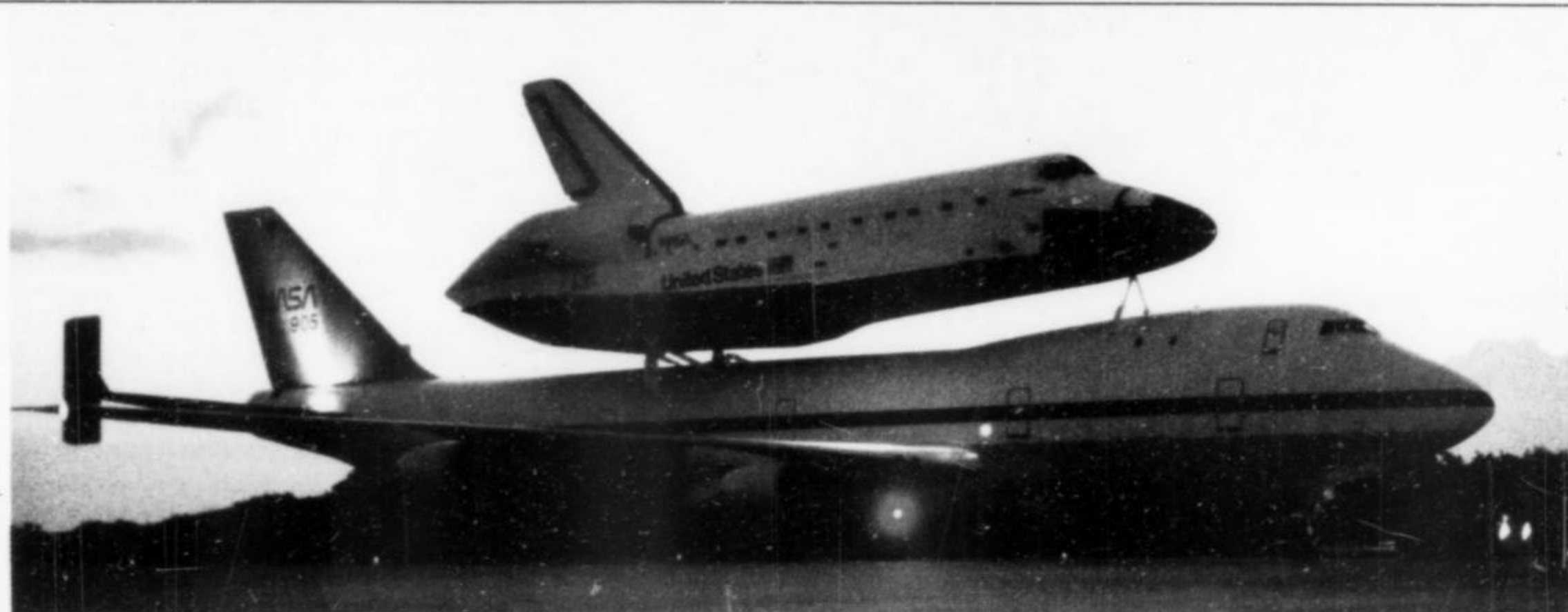
Orbiter Atlantis is shown atop the Boeing 747 carrier on its return to Kennedy Space Center following deployment of the Magellan Venus mapper on Mission 30. The orbiter will be processed to carry and deploy the Galileo Jupiter probe on Mission 34, scheduled in October.
