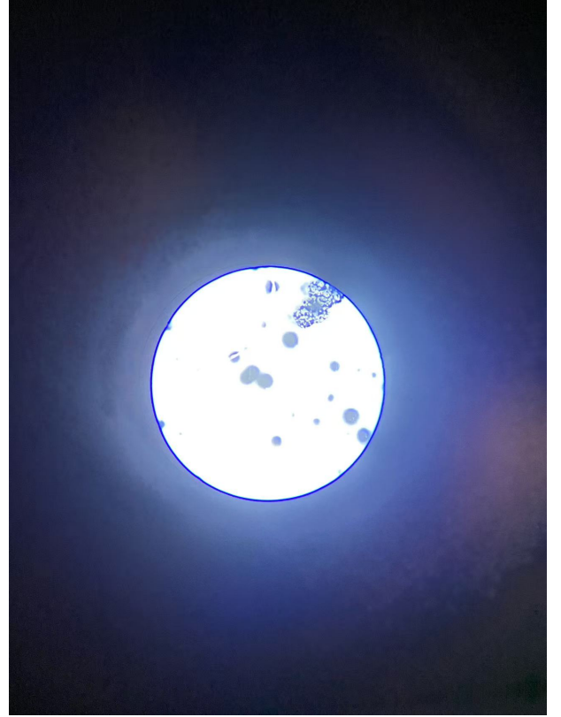
Figure 4. Microscopy image of the photographic-plate emulsion obtained from the Harvard copy plate. The bright circular region is the microscope field of view. Several compact, approximately round features are visible, consistent with stellar PSFs, together with the diffuse halo and fine grain characteristic of the copy-plate emulsion. The triple-transient candidate is present and appears as a compact, localized feature, confirming that it is not introduced by digitization. Because copy-plate grain and copying artefacts can themselves mimic compact sources ( Hambly & Blair 2024 ), the presence of the feature here establishes its reality at the plate level but does not by itself distinguish a short-duration flash from an emulsion defect; that requires comparison with the original digitization (Figure 5) and, ultimately, population-level statistics.
